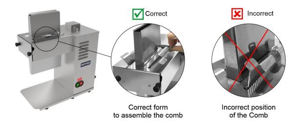
Assemble all the pieces perfectly to be guaranteed the safety of the operator and the correct functioning of the device. If any part is not firm, it may not have been properly seated. In this case, repeat the operation and not getting success, contact technical assistance.
