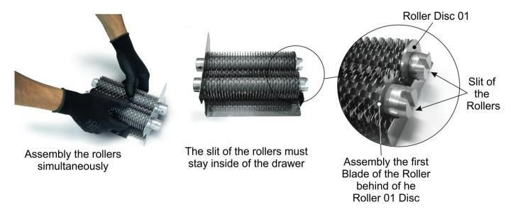
After mounting the drawer inside of the Rollers Protection, rotate the rollers until the slit fits the shoulder of the axes of the gears. To check if the rollers are properly seated, turn the knob reverse and see if the two rollers are rotating.
