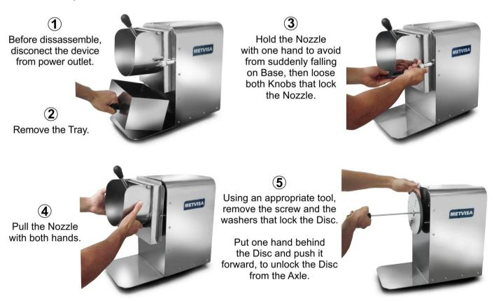
• Assembly: The assembly procedure is the reverse of removal. When remounting the Disc, choose the suitable Disc model to the process, mount it on the motor axle and turn until the Disc Notch (located behind the Disc) locks on the axle pin. Then, mount the Nozzle on the Threaded Axel (image
