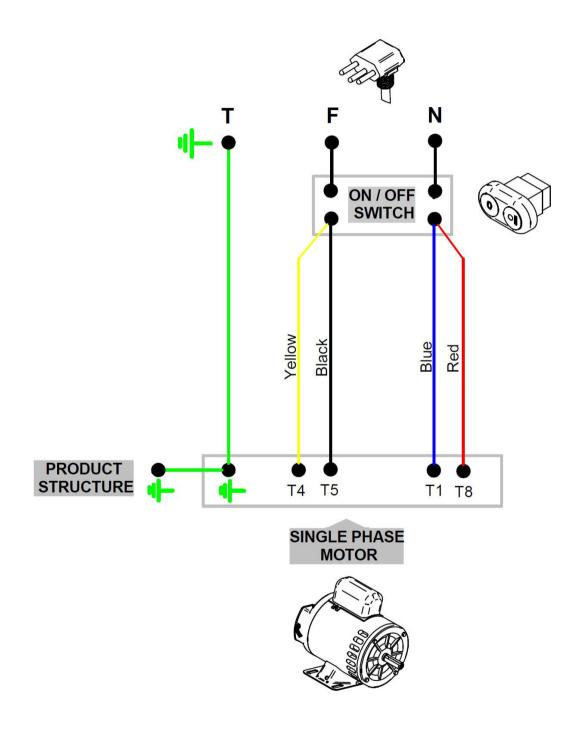
NOTE: Motor with dual direction of rotation. To reverse rotation, change T5 to T8.
