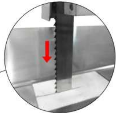
Teeth of the blade pointed down. Blade movement from top to bottom
