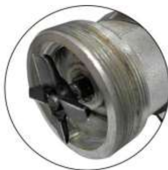
Mount the crossblade with the wire blade forward
