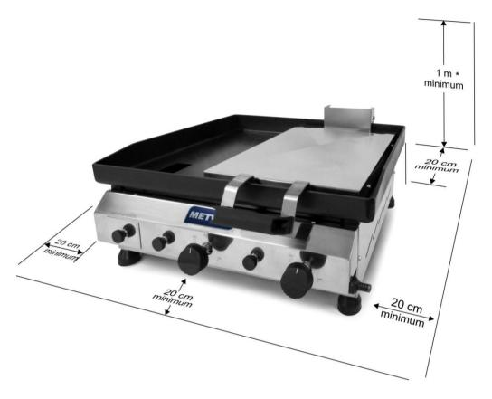
\* The minimum height measurement of 1 m was determined considering the area that the presser occupies when being lifted.
