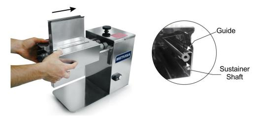
When mounting the roller in the drawer, place the slit of the rolls inside of the drawer. Note that on the roll 01 there is a disc and it should be assembly against the plate of the drawer. Another attention that you must have is regarding the first blade of the roller 02. The blade has to stay behind the disc of the roller 01, as the image below.
