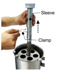
3 Lift the Bowl Protection to the screws limit and push the Beater to opposite side of the semi axis
