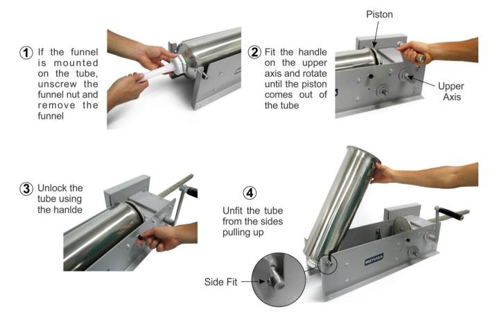
• **Assembly**: The assembly procedure is the reverse of disassembly. First assemble the tube in the slot on the sides of the equipment. Lock the tube by the handle. When reassembling the funnel, choose the funnel model that best suits the process you need at the moment, fit it in the tube, fixing it with the nut.
