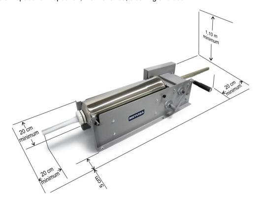
We recommend fixing the base of the sides of the equipment on a bench using screws, washers and nuts (screws, washers and nuts for fixing are not included with the equipment) so that there is no risk of the equipment moving during use.
