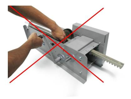
• Before starting work with your equipment, make sure that the base of the sides is fixed with screws, washers and nuts on a bench (pieces for fixing to the bench are not included with the equipment). Also check that the tube is locked with the handle.
