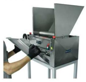
Position the holes in the table with the holes on the side of the machine;
