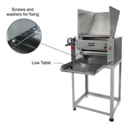
• Use the machine only for the specific products that the equipment is designated for and never put the hands, fingers or objects directly in the cylinders with the equipment on. Do not handle the dough on the side of the low table, could cause an accident.
