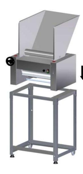
After to assembly the feet, fix the machine (CLMC.510) on the feet through the 04 screws and washers of the position 05 and 03 of the spare parts list above.
