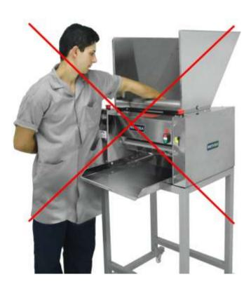
• When the equipment is being cleaned take care. Turn off the equipment pushing the on/off button and the putting general switch to the position "0" (turn off). Then, disconnect the equipment of the electrical mains. Never put the hands in the cylinders moving.
