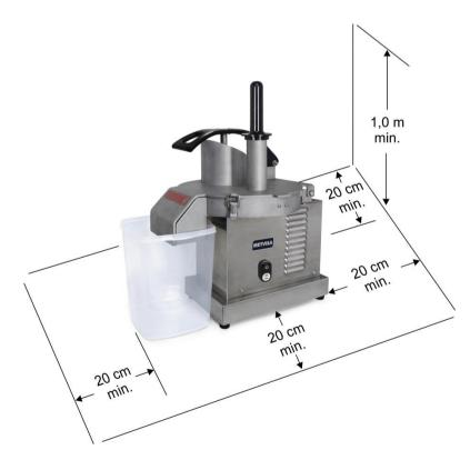
To ensure correct operation and safety, place the equipment in a well-ventilated area and on a support surface that is large enough, well leveled, dry and stable, away from heat sources and water taps, and at a medium height. of 80 cm. Install your equipment leaving a distance of at least 20 cm around it and 1.0 m in height, so that you have enough space for inspection, maintenance, cleaning and use.
