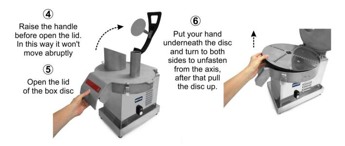
• **Disc assembly:** The assembly procedure is the reverse of the disassembly. When remounting the disc, already choose the disc model that suits the process you need at the moment. Check the disc models in item 2.1 (Main Components).
