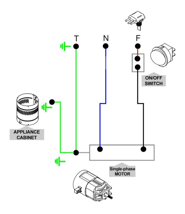
**ATTENTION:** The ground connection varies according to the type of plug. For electrical installation observe the current standards of the country, especially with regard to ground connection (if applicable).
