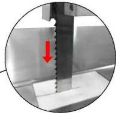
Teeth of the blade pointed down. Blade movement from top to bottom
