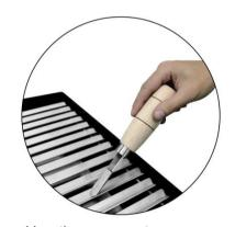
Use the scraper to remove excess of residues from the process
